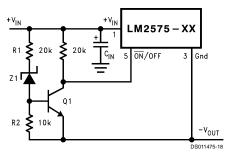
**Note:** Complete circuit not shown (see *Figure 10*). **Note:** Pin numbers are for the TO-220 package.
