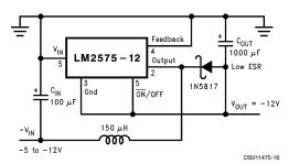
Typical Load Current 200 mA for  $V_{IN} = -5.2V$  500 mA for  $V_{IN} = -7V$
