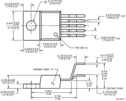
Bent, Staggered 5-Lead TO-220 (T)
