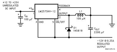
FIGURE 10. Inverting Buck-Boost Develops -12V
