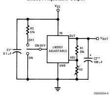
$$V_{OUT} = Reference Voltage \times \frac{R1 + R2}{R1}$$
