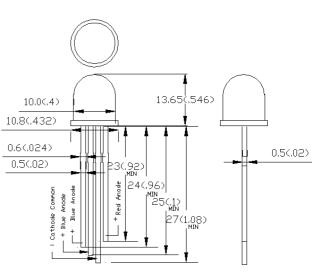
Unit: mm (inches) Tolerance: ±0.25mm (.010") max
