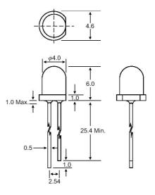
Unit: mm (inches) Tolerance: ±0.25mm (.010") max
