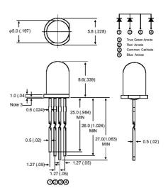
Unit: mm (inches) Tolerance: ±0.25mm (.010") max
